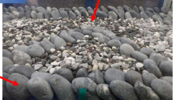
Fig. 3: Here above: The model is viewed from downstream (a). On the right: a gravel mount with stacked boulders is shown from left side wall (b).
