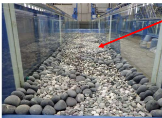
Fig. 3: Here above: The model is viewed from downstream (a). On the right: a gravel mount with stacked boulders is shown from left side wall (b).
