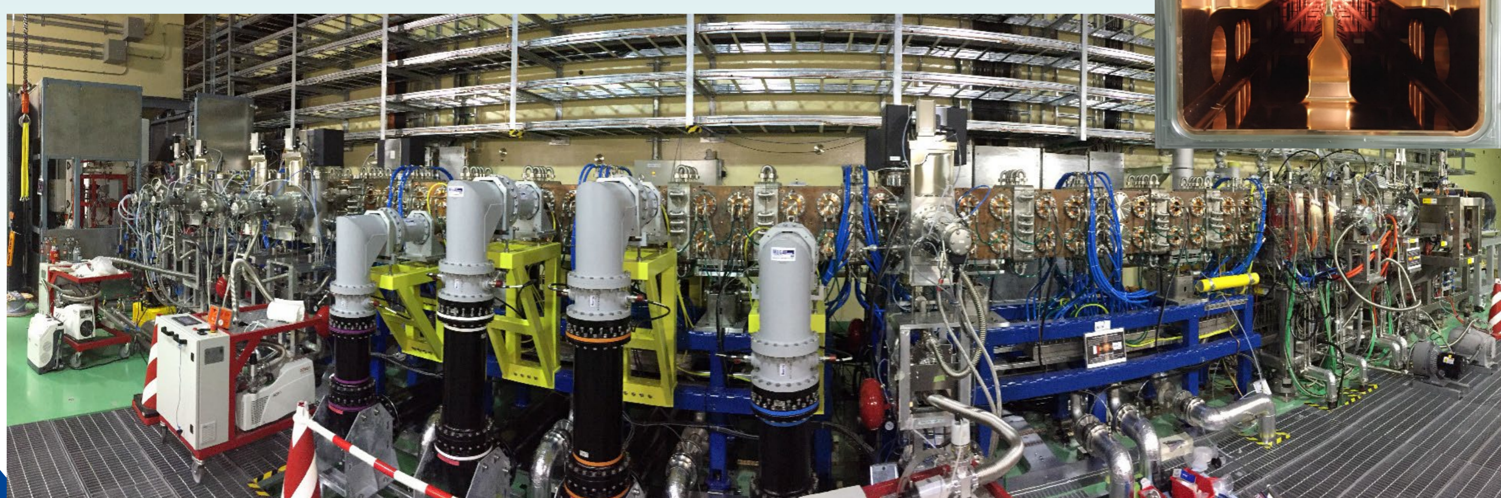
Accelerator fisheye view with RFQ at the centre; (top) internal view of RFQ
